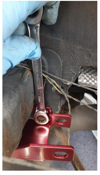
With the bar fully in place you can then use a 15MM spanner and 8MM allen to tighten the bar to the brackets. Then reinstall the bumper in the reverse order of removal.
