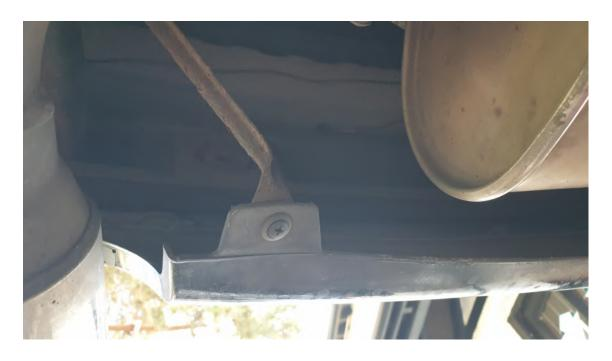
Remove the 2 7MM bolts under each brake light and pull off the bumper being careful not to drop it or scratch any paint.
